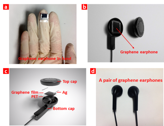
Figure 2. Graphene earphone. (a) Graphene earphone in hand. (b) View of the graphene earphone in a commercial earphone casing. (c) Exploded view of a packaged graphene earphone. (d) A pair of graphene earphones in its final packaged form.
